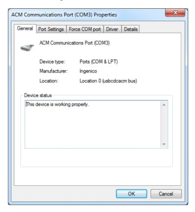
Then select the Force COM port tab to display the Force COM port features;
