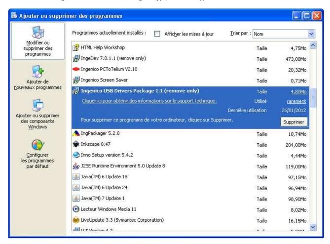
One must not try to uninstall through the device manager since it is either ineffective or incomplete. On Windows XP it has no effect and on Windows Vista and Windows 7 it doesn't uninstall the driver completely.
