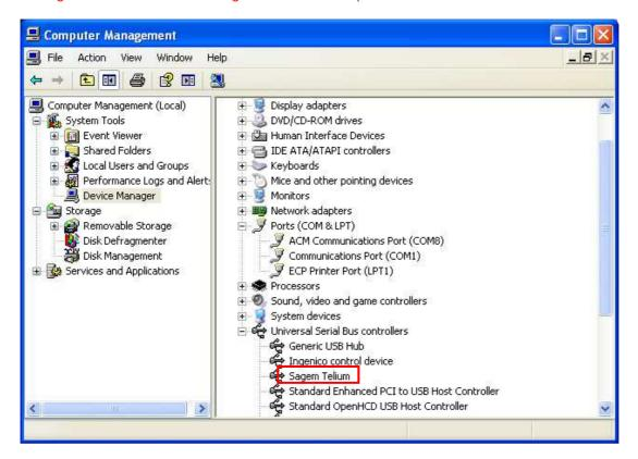
In the properties of the high-level part of the driver (the one under Universal Serial Bus controllers in the Device Manager), Right-click on the USB ID Name (eg. Sagem Telium - see section 2.1.2) and choose Update Driver and follow the instructions.
